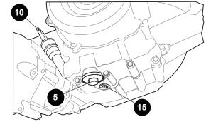
NOTICE: At the first oil change, small metal chips and lint may be found. This is normal, resulting from the break-in period. Inspect the oil screen at every oil change. The presence of large metal chips could indicate possible damage to the engine.
