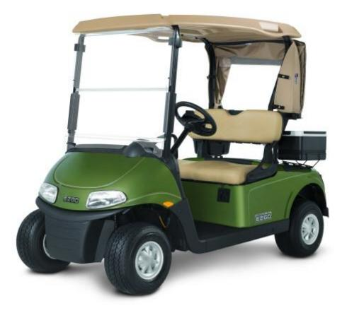
The electric RXV's patented IntelliBrake system encompasses two technologies: a motor brake that automatically slows the vehicle when travelling up or down steep grades, and a parking brake that automatically engages when the vehicle stops. This system also delivers full-time regenerative braking, redirecting energy back into the vehicle's batteries whenever the brakes are applied, recharging the batteries during use and further extending the vehicle's energy efficiency and range.
